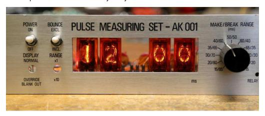
the switches for, however I will probably cut it down and lose the three rotary switches. The power switch will be power (it is to be driven by my external time source, so no need to be on 24/7), the 'bounce' switch will be a 12/24 hour display selector, leaving the bottom two hole for time set buttons - not needed at my QTH, but handy for demoing it at a club meetings etc.
