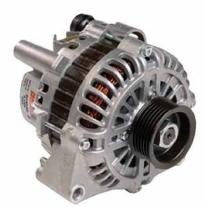
control that will vary the output between 12.3V and 15V depending upon conditions (and internal whim) The Range Rovers, Nissan Navara's & Pathfinders, Pajero's Land Rovers and Mazda's now do this. The car computer will turn down the alternator charging if it thinks that the battery ought to be charged, or if the engine is idling, or if the driver is accelerating. I'm sure that drivers can really feel that 2% energy boost pushing them harder into the upholstery as they power away at the lights.
