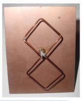
ple is similar. Each segment is 62mm from center to center (bend to bend), with the antenna ~ 30mm off the reflector. If you wish to support the antenna top and bottom, then a high value resistor could be used.
