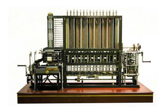
Charles Babbage's Difference Engine No. 2, designed in the late 1840s, weighs five tons, is 11 feet (3.4 meters) long and seven feet (2.1 meters) high, and has 8,000 bronze, cast iron and steel parts. The Computer History Museum's Babbage Engine Exhibit launches on May 10, 2008, in Mountain View, Calif.
