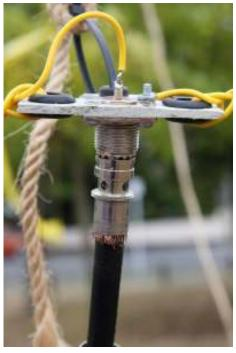
iron was produced, with thanks to ZL1TNO, and the connection to the SO239 repaired. The feeder was replaced, with the suspect feeder taken away for later repair, with thanks to ZL1IC.
